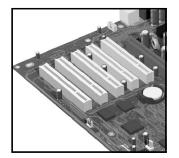
The PCI slots accept 3.3V and 5V PCI 32-bit 33MHz cards, and Universal PCI cards (which are 3.3V or 5V compatible). Refer to the table on page 34 for the different PCI board installations.
